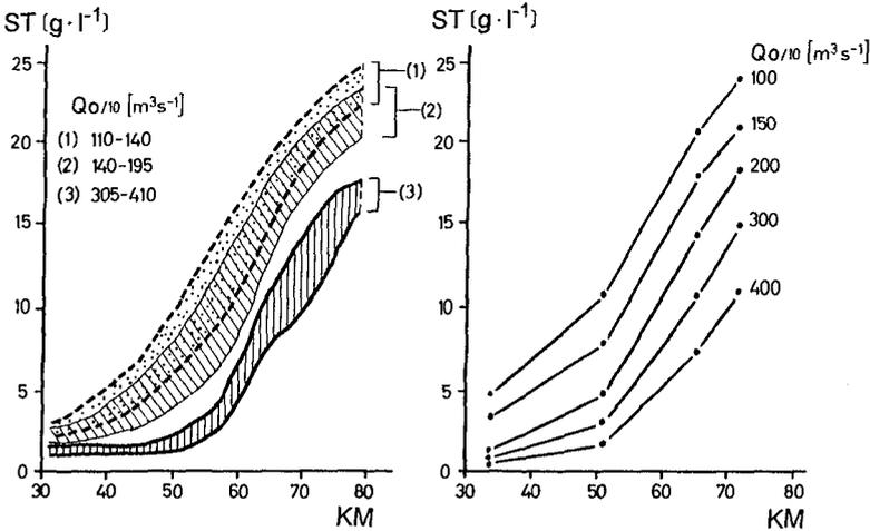
Fig. 10 Longitudinal profiles for Total Salinity (ST) as function of ( $Q_0/10$ ). Left: envelopes for groups of measured profiles. Right: ST-functions ( $Q_0/10$  is parameter) calculated with measured profiles
