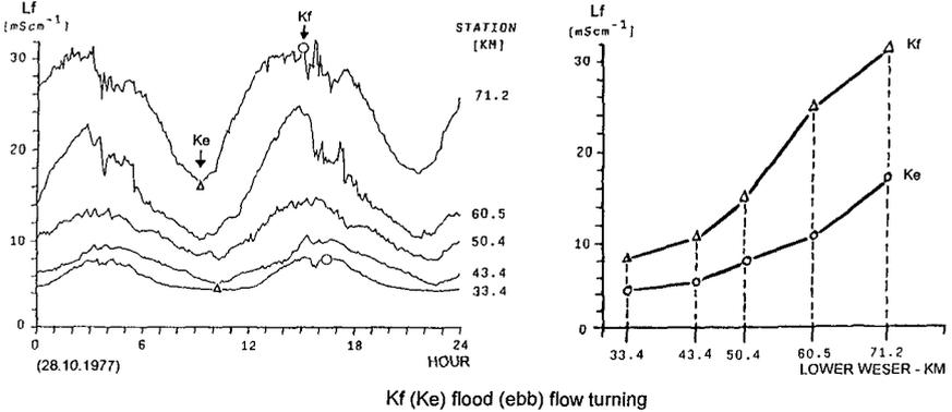
Fig. 9 Left: Conductivity ( $L_f$ ) over time for different measurement stations in the Unterweser. Right: Conversion of the  $L_f$ -data into longitudinal  $L_f$ -profiles for the tide phases Kf and Ke (KUNZ 1979)
