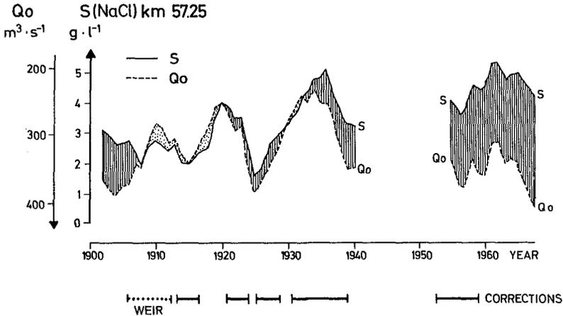
Fig. 13 Combination of Salinity S (NaCl) for Nordenham (km 57.25) with the Run Off ( $Q_0$ ) at Intschede-gauge after STRÖHMER (1970)
